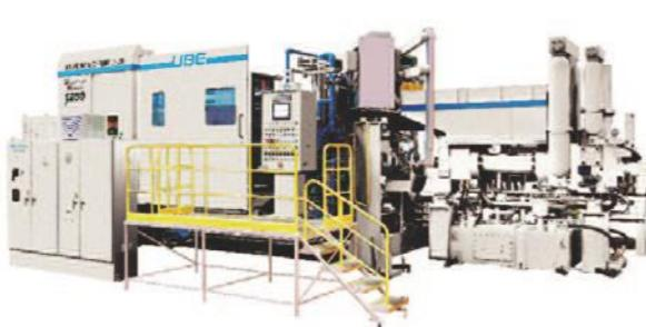
Two platen hybrid die casting machine : UH Series
